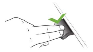
Figure 2: Press and hold the DPG to make the desk drive down
