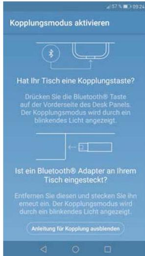
To get a functional app, you must have the LINAK Bluetooth® Adapter or desk panel with integrated Bluetooth® DPG1B . The screen to the left informs the user how to get the product they received in pairing mode.
