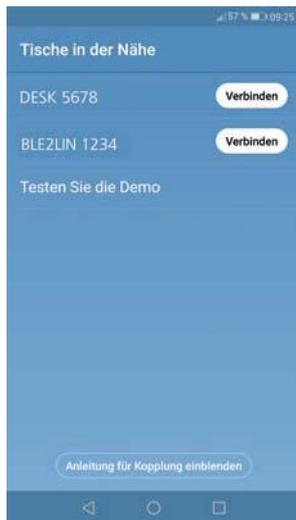
When pressing “Hide pairing guide” the screen with the list of devices in pairing mode will appear. Press the “connect” button to the right of the device to pair.
